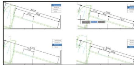
The DIM command remains active until you exit the command, so you can knock out multiple dimensions at one time.
